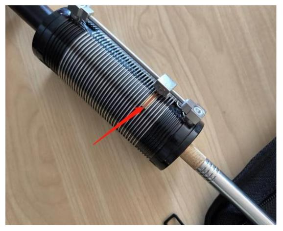
21.4MHZ with 4 sections of aluminum tube + 7 sections of antenna whip+ 10cm, SWR1.1-1.3
