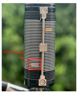
**b. 20-meter band:** The position marked by the red line at the upper end of the coil.
