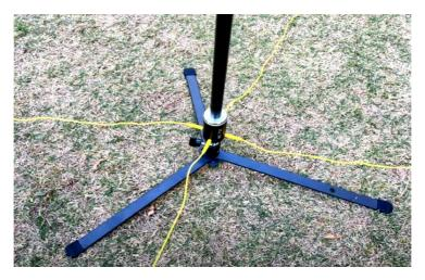
To better protect threads for the antenna base, it is recommended to use the tripod with the supplied 2 adaptors connected together and the MC-750 or JPC-12 antenna connected to the M10 end of the adaptor. However, the 1/4 to 3/8 adaptor can also be used directly with the antenna.
