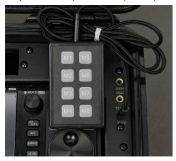
Memory numbers 1 to 8 can be recalled for CW, RTTY and SSB modes.
