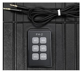
• Press the "MEM" button in the lower right corner and the 'REC' will flash on the screen. Then press and hold the #1 storage button, then press the PTT button to record the first audio.and the 'REC' disappears to indicate that the recording is complete.
