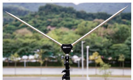
There are reference marking points printed on the whip antenna. Adjust the length of the whip to meet your desired frequency according to the reference marking points. (All sections above the mark needs to be fully extended and all sections fully collapsed... The 7MHz band requires the use of the wire elements provided above.)
