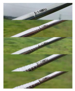
Although there are reference points, you might still need to do fine adjustments to the length of the whip antenna until you get a sensible VSWR readings(From an in/external VSWR meter, VNA or antenna analyzer).
