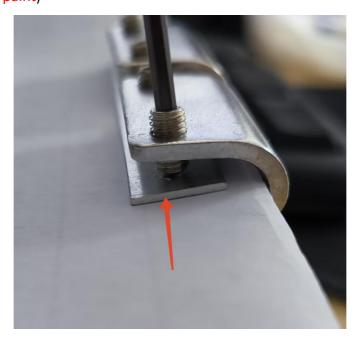
Attach the antenna connector to the mount (Note that you can use the large handle to adjust the tension at the indicated position)
