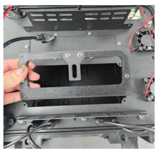
3. Install the front panel of the radio FT891 into the slot of the metal panel.
