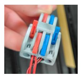
9. Install the power cords:Note that the two power cords of the main unit should not be exposed at all, otherwise it will cause a short circuit
