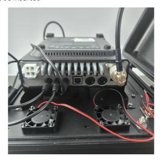
8. As shown in the picture, open the power buckle and connect the power cord of the main unit
