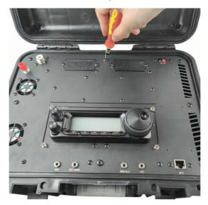
11. After fixing the metal panel, you can also install the hand microphone according to your needs.
